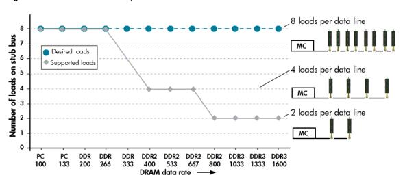
Figure 11. Maximum number of loads per channel based on DRAM data rate
