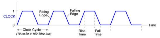
The clock cycle time is measured in nanoseconds (ns,  $1 \times 10^{-9}$  second) and the clock frequency is measured in megahertz (MHz, millions of cycles per second). The clock frequency is the reciprocal of the clock cycle time. For example, if the clock cycle is 10 ns then the clock frequency is 1/(0.00000010)=100 MHz.
