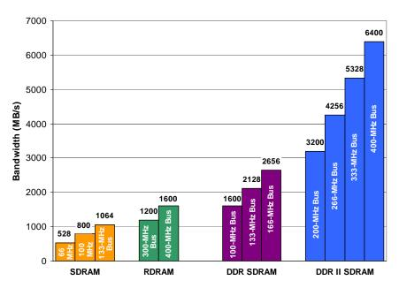
Figure 8. Peak bandwidth comparison of SDRAM and advanced SDRAM technologies
