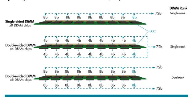
Figure 7. Single-sided and double-sided DDR SDRAM DIMMs and corresponding DIMM rank
